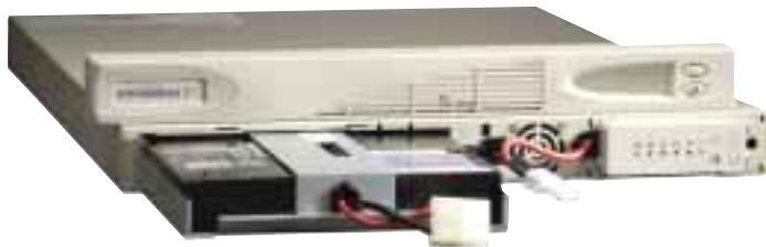
Powerware 5115 RM shown with front cover removed and battery sliding out.
